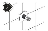
Screw the **Bottom Trim** on to the adaptor so that it sits flush to the wall.
