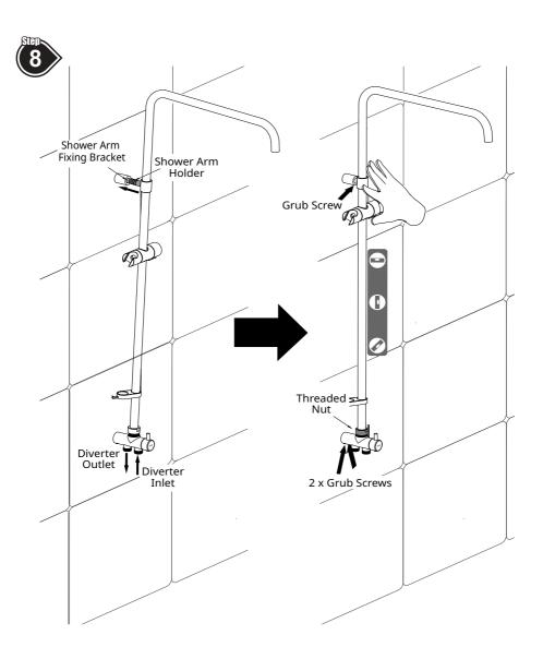
Pivoting the **Shower Arm** slightly away from the wall, slide the stem of the **Shower Arm Holder** into the **Shower Arm Fixing Bracket**.
