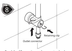
Feed the 15mm pipe and connector back up the Riser Rail and secure the Outlet Connector with the Retaining Clip. Fit the Bracket End Trims onto the Brackets.
