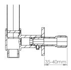
Screw the **Adaptor** to pipework.
