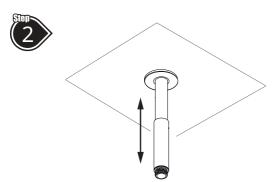
When the pipework fitting is secure and the ceiling is made good, carefully screw the **Ceiling Arm** onto the fitting.
