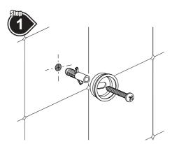
Mark the wall fixing position for the **Diverter Fixing Bracket** and drill and plug the wall. Ideally the hole should be positioned in the centre of a tile and not in the grouting.
