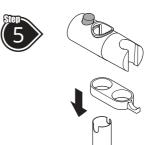
Slide the **Hose Retainer** and then the **Shower Head Holder** onto the **Riser Rail** — press and hold the button on top of the holder to release the locking mechanism, then slide onto the rail.
