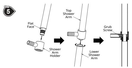
Assemble the **Top Shower Arm** into the **Shower Arm Holder**, note that the **Top Shower Arm** can only be assembled one way, so ensure that the flat faces of **Top Shower Arm** and **Shower Arm Holder** are aligned.
