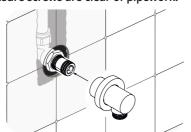
Fit the **Bulkhead** onto the **Adaptor** and retighten the grub screws.
