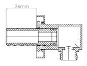
Screw the **Bulkhead Adaptor** to the pipework. Add a bead of silicone sealant around the adaptor to ensure watertight.
