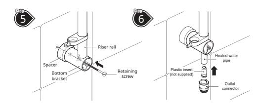
Secure the **Riser Rail** and **Bottom Bracket** assembly to the wall using the supplied screw.
