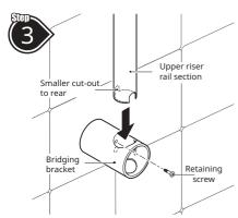
Measure the 940mm rail (for the upper section of rail) and mark the required length to fit between the **Bridging Bracket** and into the ceiling.
